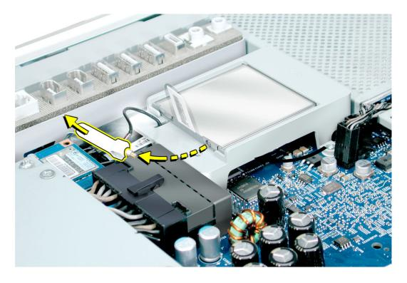
5. Pull the tab on the card to remove the card from the AirPort card guide.
